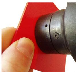
For **plastic identification** the sparking head is simply pressed on to the analysis sample. The measurement begins by pressing the start button on the pistol grip. After one second an integrated LCD displays the result. Furthermore the result can be shown on an external VGA screen
