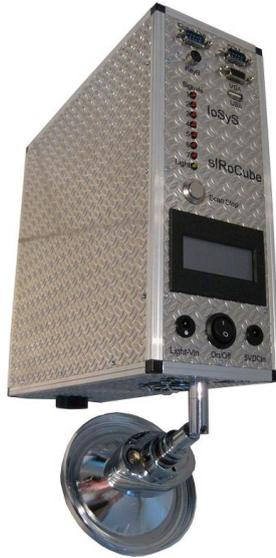
The **basic principle** of the method is the diffuse near infrared reflection spectroscopy whereby characteristic absorption behaviors of different polymer types are used in that spectral region. The polymer sample is radiated with a infrared light and the reflected light of the measuring place is analyzed using a near infrared detector array.
