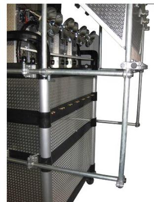
As modular system **sIRoSort**, several sIRoCubes can be combined in parallel, equipped with a controlled pressured-air ejection array to eliminate unwanted plastic types (e.g. PVC) like for the **separation of PET bottles**. The unit with adjustable feeding funnel and a roll-on cart is simply placed under a conveyor belt which transports the input feed of mixed plastics.
