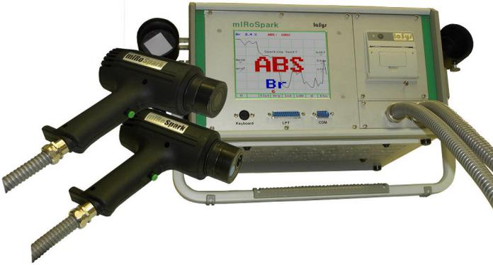
With this technology combination **practically all common types of plastics, regardless of color, size, structure** (films, foils, granules, solid, foamed, carpets and textiles) can be identified together with their additive elements like **fire retardants** and **heavy metals**. For sample preparation to remove dust and dirt or paintings the sample surface can be easily cleaned by scratching with a knife.
