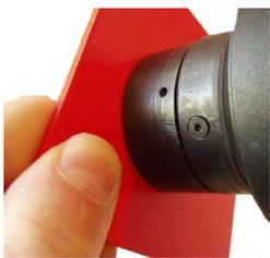
For **plastic identification** one of the measuring pistols is simply pressed on to the analysis sample. The measurement begins by pressing the start button on the pistol grip. After one second an integrated color TFT-screen displays the recognized polymer. The measuring pistols are connected with a 2 m cable each to the instrument. The optical signals
